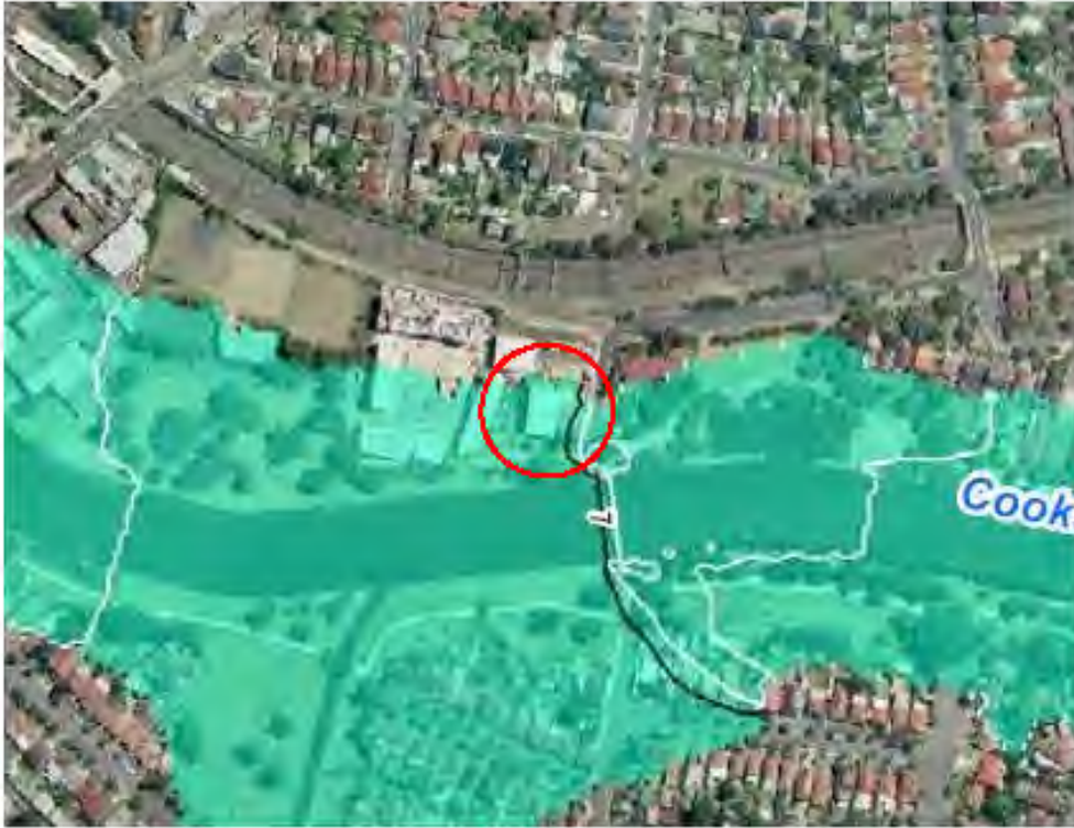
Image 6.11. Map picturing a probable maximum flood (PMF) event associated with climate change. This shows the water level flooding the Sugar House. (Sydney Water, 2009, Annexure B, Figure B31)
