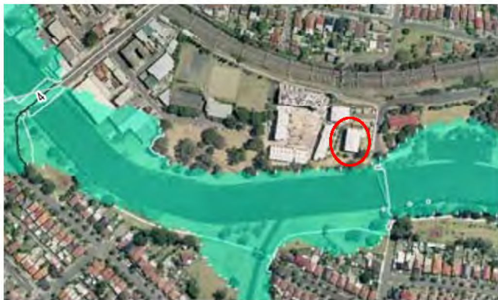
Image 2.4. Map picturing a 100-year flood event shows the water level covering the pedestrian pathway but not reaching the ground level of the property. (Source: Sydney Water, 2009, Annexure B, Figure B17)
